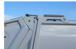
2 Tailgate lift cylinders on the hopper roof
