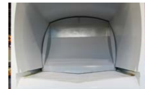
1 Leachate tank at the bottom of the body Keel shaped floor helps leachate flow to drain sump
